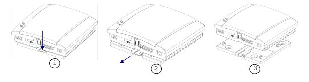
2. Fix the wall-mounting bracket on the wall.
